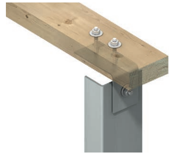
Top Connection of a WP2 Windpost to the Underside of a Timber Wall Plate
