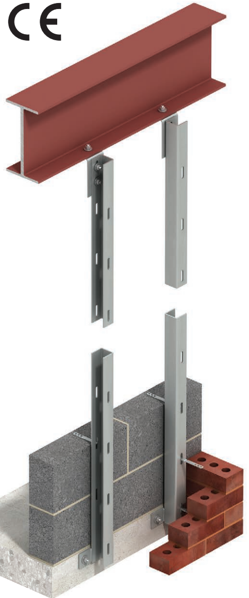
WP3 Fixed to Concrete at the Base and a Steel Beam at the Top
